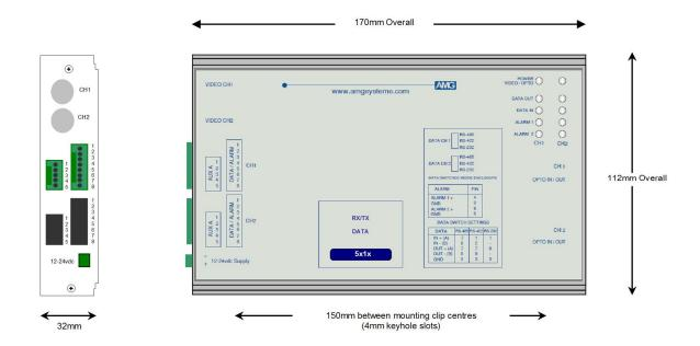
The **AMG5414A9** is a standalone receive unit designed to transmit & receive one Bi-directional alarm, one Bi-directional audio channel and one Bi-directional data signal over a Singlemode optical fibre.
